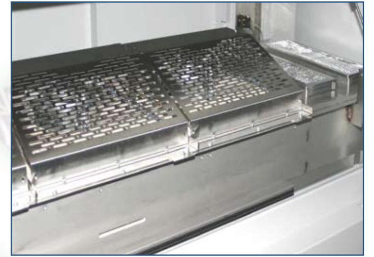
Photo: Heating cell with cooling zone
